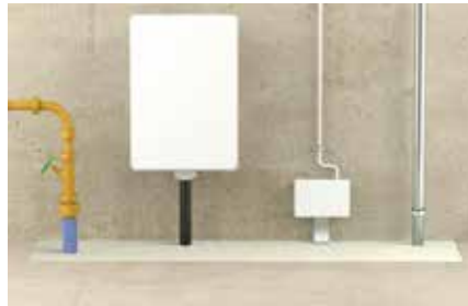
Mixed penetration through the floor
