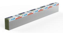
For use in open state cavities within the external building facade where continuous ventilation and drainage is required. Silverliner incorporates a foil lined mineral wool fibre board with a high-performance intumescent strip, so in the event of a fire the intumescent strip quickly swells to close the gap, slowing the spread of smoke and flame around the outside of a building.
